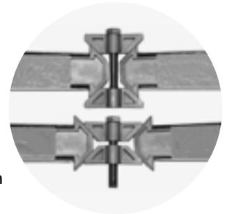
Depending on the diameter of the pipe joint being sealed, there will be between one and four WedgeLock Assemblies on each expansion band to ensure an even distribution of compressive force on the rubber seal.
