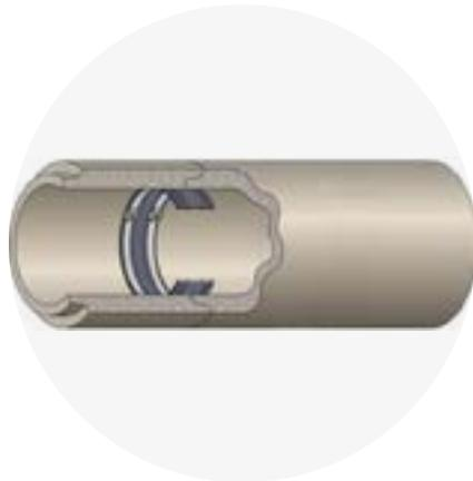
The compressive force providing the seal on either side of the joint is the result of increasing the effective diameter of the stainless steel expansion bands.
