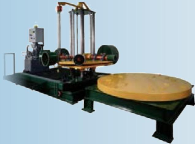
Hydrokor III is made for the large volume producer who needs to quickly and efficiently core drill several different hole sizes.
