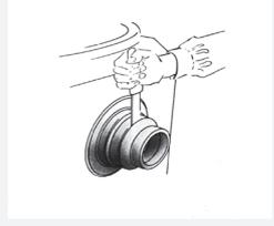
Place the seal in the hole and tap it into the correct position using a rubber or plastic mallet. Tap the end of the short plastic supporting that is fitted in the seal
