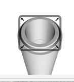
The seal must sit evenly against the spigot shoulder all around the manhole. Lubrication of the socket or spigot is not required.
