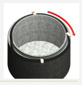
Equalize the stress in the seal by lifting and releasing at a few points.
