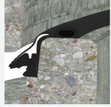
Centre the joint assemble. The position of the seal in the final mahole joint is shown. If re-joining is required ensure the sliding skin is drawn back to the position as shown in Figure 1.
