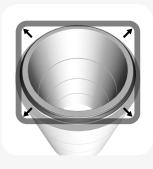
Equalize the stress in the seal by lifting and releasing at a few points. The seal must sit evenly against the spigot shoulder all around the manhole.
