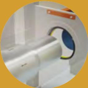
The seal is automatically loaded on the socketing mandrel against the support flange
