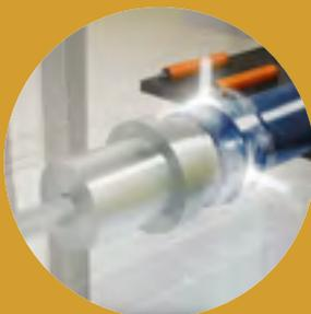
The pipe socket is cooled either by air or water and the mandrel withdrawn from the socket
