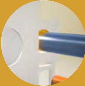
The pipe is heated to allow forming of the socket
