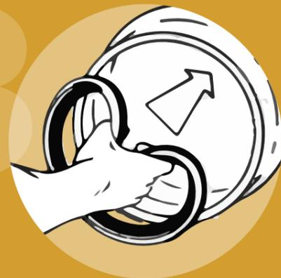
Insert the seal into the socket of the pipe and press the seal out into the groove. Ensure the seal is located correctly
