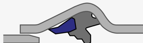
Immediately after lubrication, the spigot should be brought into contact with the socket.
