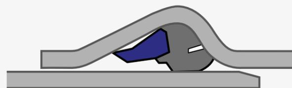
Both spigot and socket should be correctly aligned and then slide the spigot into the socket, thus compressing the seal until the joint is fully made.
