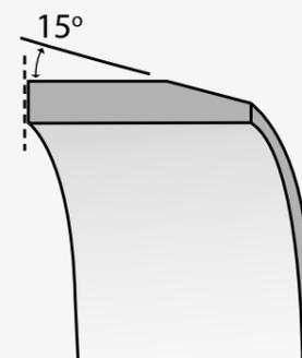
The pipe spigot should be chamfered with an angle of 15°, taking care to remove all burrs.
