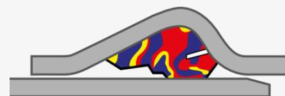
When two pipes are pushed together the rubber sealing element is designed to deform creating a sealing pressure acting on both spigot and socket.
