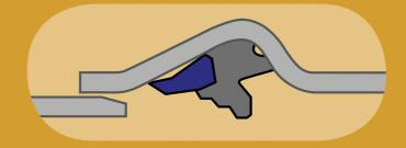
Apply lubricant to the spigot end and immediately bring it into contact with the socket
