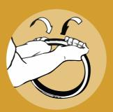
**Locate the bending zone of the seal**
