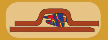
When two pipes are pushed together the rubber sealing element is designed to deform creating a sealing pressure acting on both spigot and socket.
