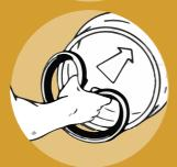
Insert the seal into the pipe and press the seal into the groove
