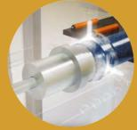
The pipe socket is cooled either by air or water and the mandrel withdrawn from the socket
