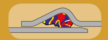
By compressing the sealing element, the EPDM rubber will deform and create pressure on both spigot and socket. This results in a watertight seal.
