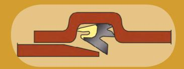
Apply lubricant to the spigot end and immediately bring it into contact with the socket
