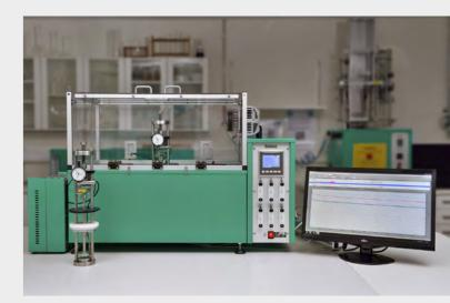
As per the ISO guidelines, a maximum relaxation level of 50% was set and Elastocon estimated the number of years the elastomeric material in the seal will take to reach the threshold. This test has proven that Trelleborg compounds for pipes seals offer **eight times the service life** of competitor systems.
