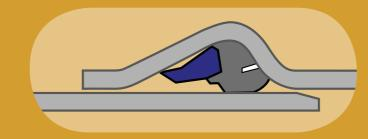
Align spigot and socket, and slide the spigot into the pipe, past the seal
