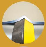
The support flange is retracted, and internal vacuum and external pressure forms the pipe around the contours of the seal
