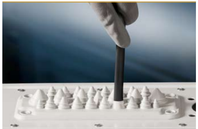
Pull the cable or tube back some 20 mm to lock it.
