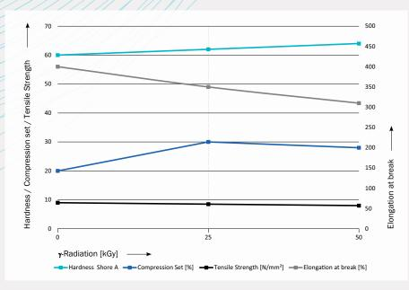
Figure 3: Physical behavior of silicone during Gamma sterilization. Changes at physical properties can occur due to Gamma Sterilization.
