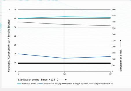
Figure 1: Physical behavior of silicone during steam sterilization.
