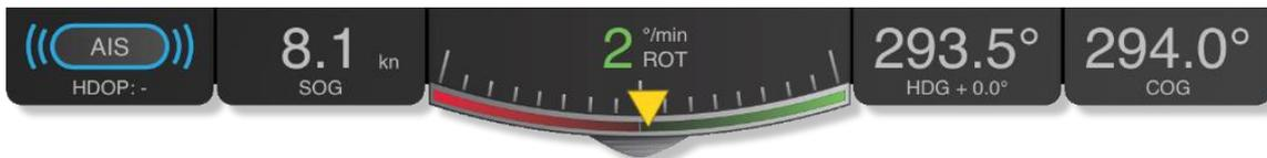
The heading can be adjusted by tapping on the HDG and entering the correction.
