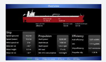
Data collected by a shaft power meter can be useful in measuring efficiency and saving fuel and emissions (source: Trelleborg)
