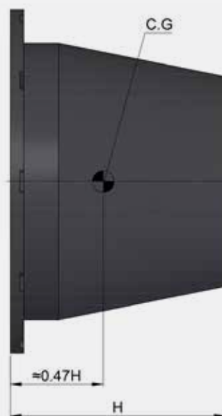
Figure 3 – C.G detail of SCN Fender
