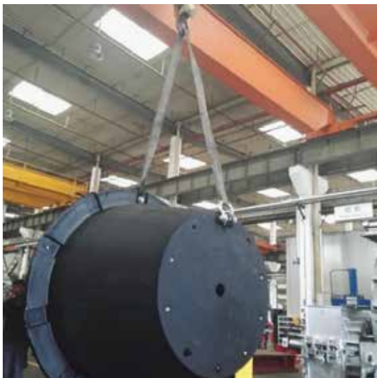
Figure 1 – Fender lifting using crane hook
