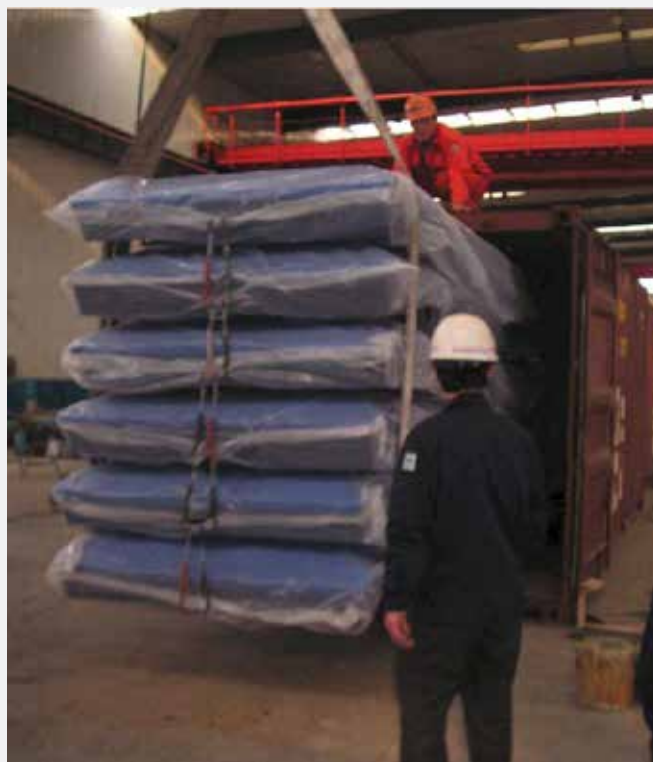
Handling (unloading) frontal frame using crane
