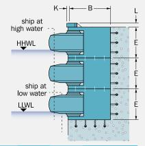
The table indicates typical Wheel Fender casing dimensions. For special applications and unusual corners, the casing shape can be altered for a perfect fit. Please ask Trelleborg Marine and Infrastructure for details.
