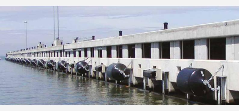
Used in a variety of challenging applications, foam fenders are extremely versatile. Easy to install, they provide a tough, heavy-duty fender solution for in-harbor, off-shore and ship-to-ship applications. Their resilient foam-filled construction provides an unsinkable fender body that permits high energy absorption with relatively low reaction force and low hull pressures.
