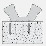
Retrofit Mounting Type (using EC 2 epoxy anchors)
