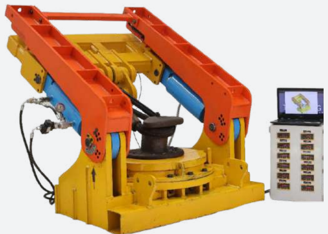
BOLLARD TESTING MACHINE
