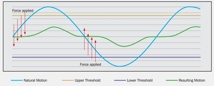
Note: Mooring forces applied by AutoMoor reduce the peak mooring loads resulting in a flatter vessel motion curve.
