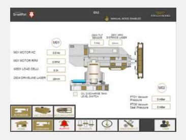
AutoMoor is SmartPort enabled, with data logging and reporting available on multiple levels. SmartPort by Trelleborg is a technology platform that connects port operation systems, allowing users to analyze the performance of assets and apply data insights to identify optimization and efficiency gains.
