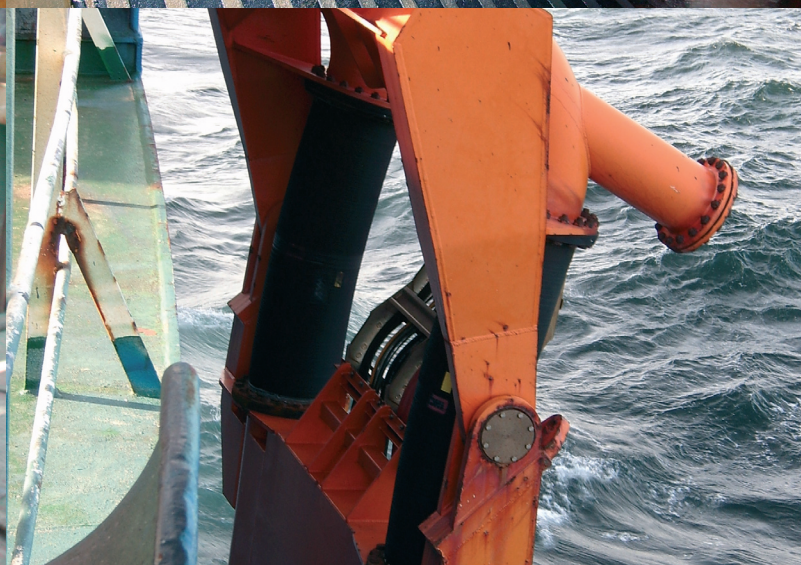
▲ Jetwater hose on service frame
