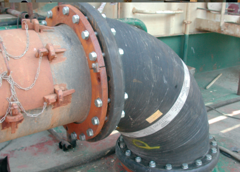
▲ Preshaped rubber elbow in loading line gravel dredger Rubber elbow gives a long service life
