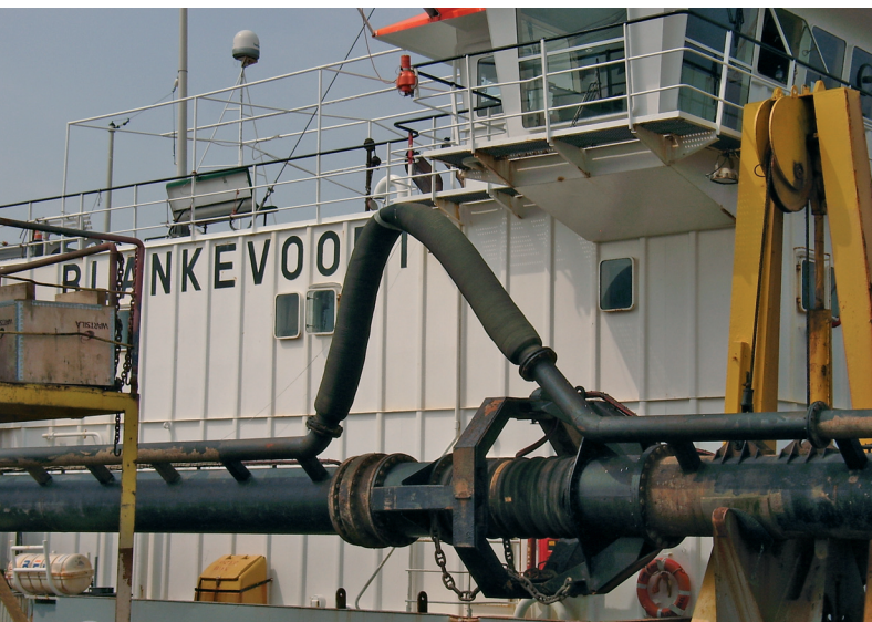
▼ Jetwater hose over gimble joint This replaces 3 hoses + 3 bends
