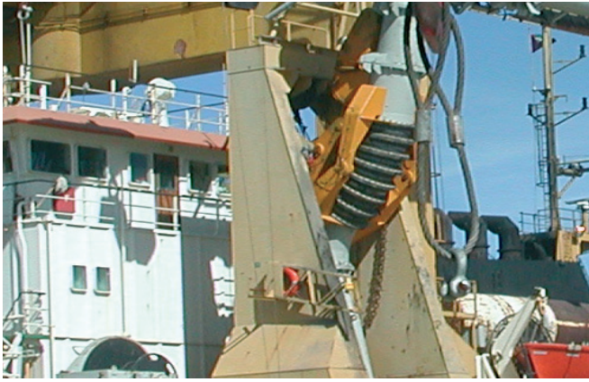
◀ Bucket hose in barge loading line cutter dredger
