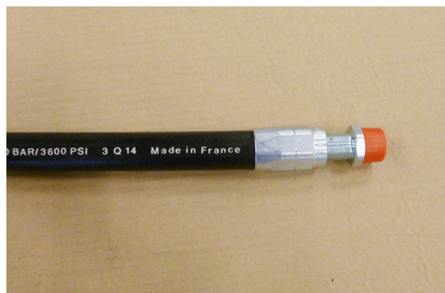
Skruva nippeln i hylsan. Start to screw the nipple into the ferrule.
