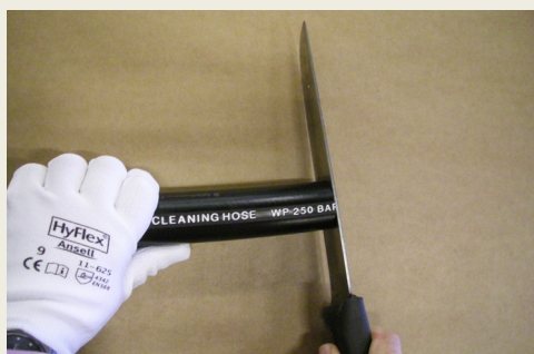
Kapa slangen helt rakt. Cut the hose perfectly straight.
