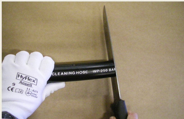
Kapa slangen helt rakt. Cut the hose perfectly straight.
