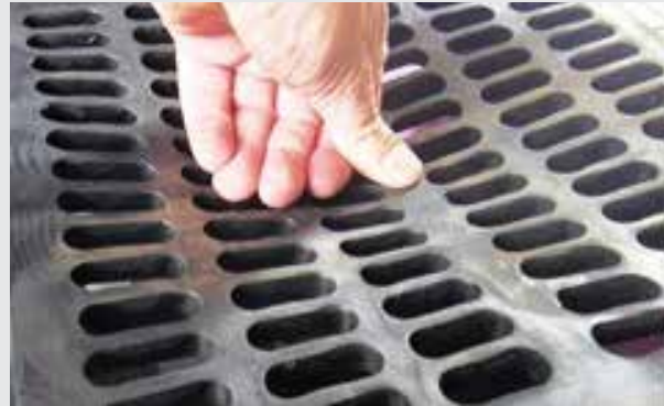
Under 20kg load, a 50mm deflection
