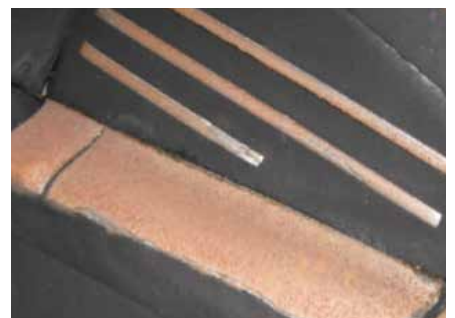
Trelleborg MillTough™ extreme lifter bars, along with MillTough™ extreme head plates, (head plates are twice the life of lifters).
