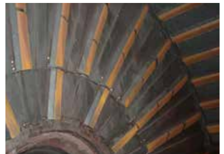
Trelleborg MillTough™ extreme lifter bars, along with MillTough™ extreme head plates, (head plates are twice the life of lifters).
