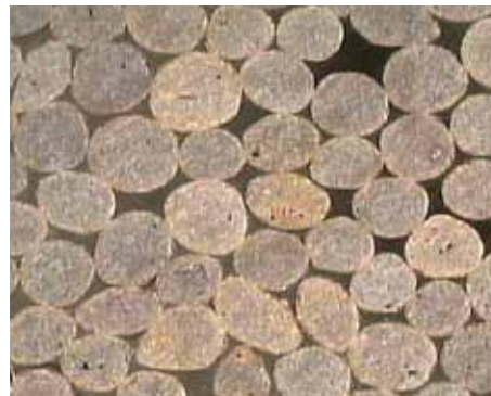
TESAEpoxy Ceramic Bead – 20x Magnification
