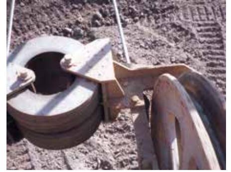
MODIFIED View shows simple method of replacing spacer bar with bolted frames and buffers held by long bolts.
