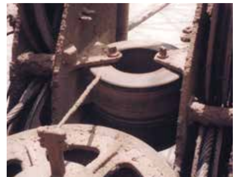
Simple on site modification by the addition of three plates to each Sheave housing, with long bolt fasteners. These buffers have been in service since their installation and display no signs of damage or deterioration.
