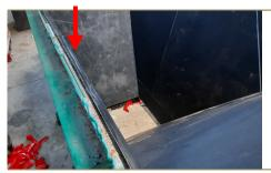
Introduce a tool as a lever at the edge of the rubber to lift it up carefully
