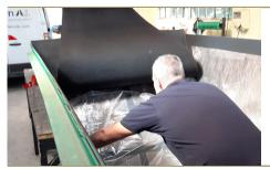
Remove the plastic layer protecting the Hookgrip surface.
