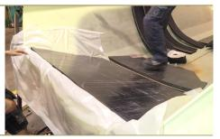
Then, place the rubber plate on the top to confirm that dimensions are correct.
