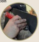
Once pressure has been applied, a short exposure to heat, ~ 2 minutes of hot air at 60/80°C (140/176°F), can intensify the bonding effect.
