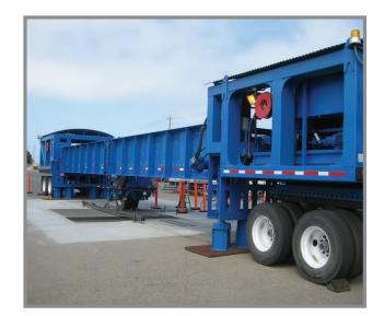
HVS testing on the deck joint
