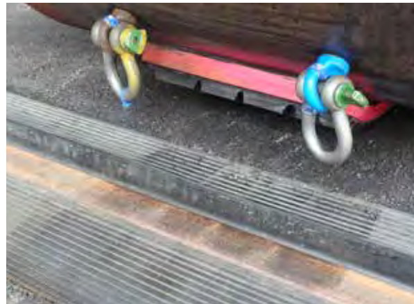
Static load test at 3.5 Tons
