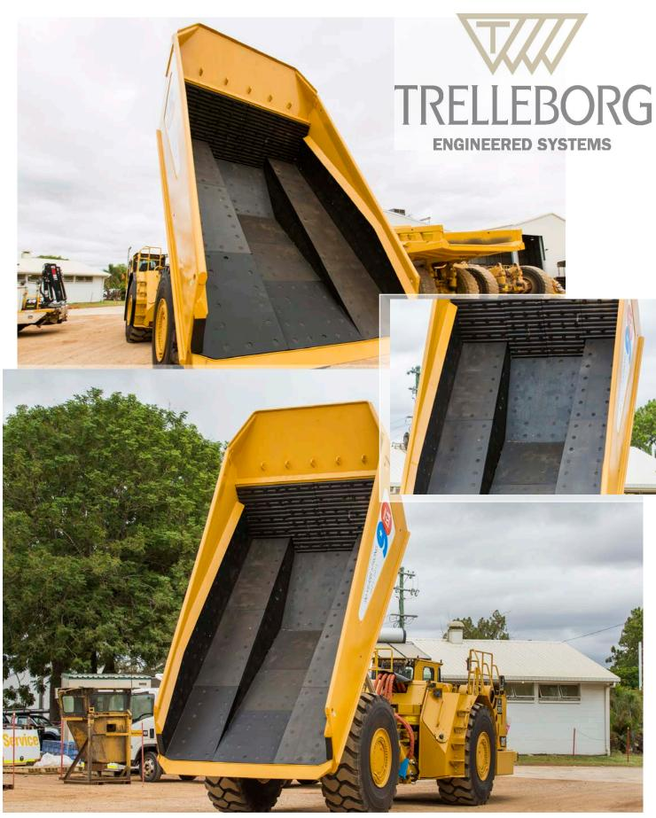
Trelleborg – High Impact and abrasion rubber wear liners were installed in a Caterpillar AD 45 B dump truck body. These dump Trucks carry ore from underground to above surface. Trelleborg Liners reduce carry back but protect the truck body from aggressive wear, improve OH&S, and allow the mine improved availability due to reduction in maintenance downtime.
