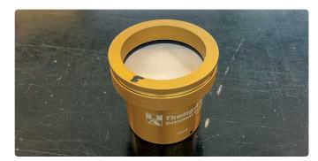
A piece of fabric from each product range, (PER200, MIC861, MIC+406) were cut to size and placed over the testing apparatus and was filled with 108ml of distilled water.
