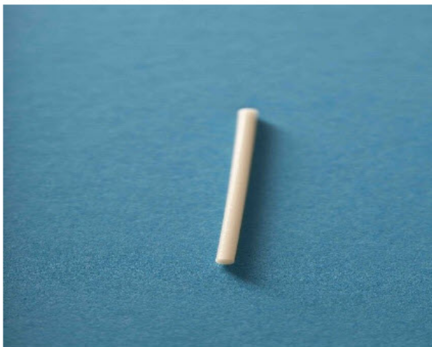
Figure 4: Silicone is an ideal material for combining with an API and creating an implanted drug reservoir.
