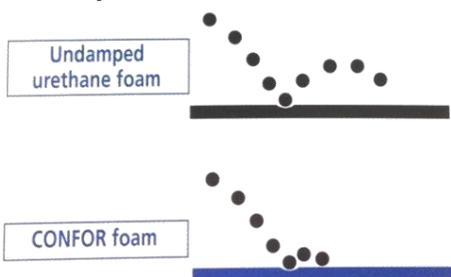
An undamped urethane returns nearly all of the impact energy, while Confor® foam absorbs it.
