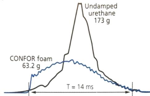
A 16.9-pound weight is dropped from a height of 2 feet onto 1-inch-thick materials. This demonstrates Confor® foams' energy-absorption capabilities. The peak acceleration response registers 173g with an undamped urethane foam, but only 63.2g with Confor® foam.
