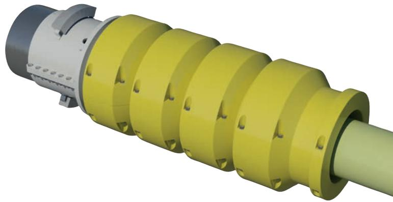
Once the elements lock together the bending moment present is transferred through the elements to a specially designed steel interface structure then into the adjacent rigid connection. To provide the performance at every level, Trelleborg Offshore will design the bend restrictor elements based on supplied information and configure the termination steelwork to suit the project needs.
