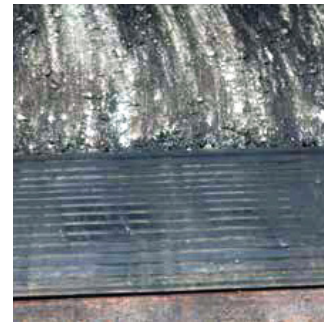
After 10 passes at 3.50 Ton Dynamic test
