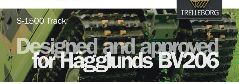
Trelleborg's Applied Technologies well-proven S-1500 track is designed and approved according to Hägglunds specification for BV206 tracks.
