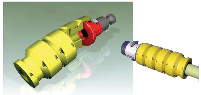
Once the elements lock together the bending moment present is transferred through the elements to a specially designed steel interface structure then into the adjacent rigid connection. To provide the performance at every level, Trelleborg Applied Technologies will design the Njord BR elements based on supplied information and configure the termination steelwork to suit the project needs.
