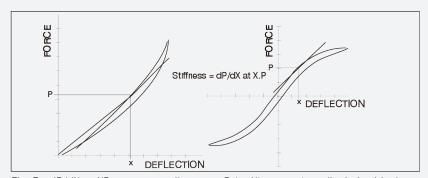
Fig. 5. dP/dX at XP average gradient over P (or X) range (usually derived by least squares method of curve fitting).
