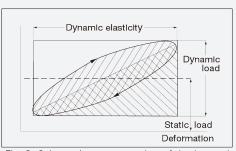
Fig. 3. Schematic representation of the internal damping properties of rubber. The elliptical area indicates the loss of energy.
