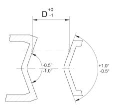
**Tolerances**Tolerances at the adjoining faces should be as shown
