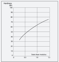
Fig. 11. Relationsip between rubber hardness and shear modulus.
