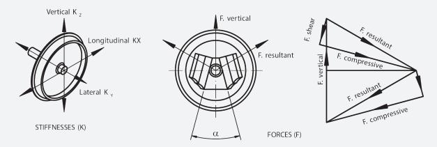
The three modes of flexibility for axlebox suspension are shown here. Springs are fitted inclined at an angle to the vertical axis, loading the rubber layers in shear and compression.
