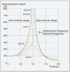
Fig. 2. Resonance curve for spring material with different internal damping.
