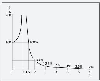
Fig. 13 Resonance curve.
