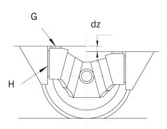
The vertical deflection (dz) may vary due to creep, Gough-Joule effect and stiffness tolerances. Shims (G) should be included for height adjustment. Shims (H) are sometimes necessary for accurate alignment of axles.
