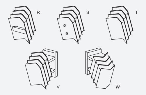
Springs can be supplied with alternative methods of location as shown in the diagram, namely with cross bar (R), dowel pins (S), or edge location (T). Location on the bogie frame is normally on the plate edge. Springs can be supplied with brackets for direct and easy fitting to the bogie frame (ref . figs V & W)
