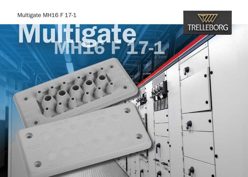
Multigate MH16 F 17-1 is a new plastic reinforced cable gland suitable for leading through cables and various types of tubing. It matches the cut out dimensions of 16-pole standard industrial connectors. No separate gasket is needed.
