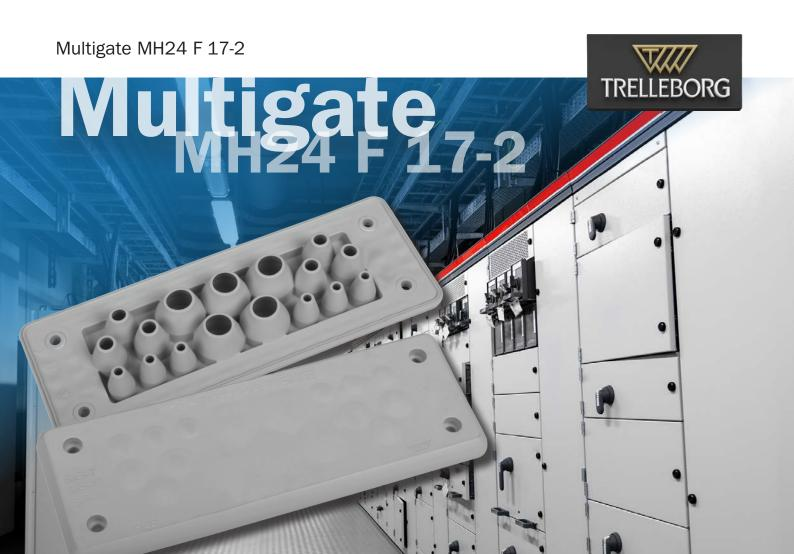
Multigate MH24 F 17-2 is a new plastic reinforced cable gland suitable for leading through cables and various types of tubing. It matches the cut out dimensions of 24-pole standard industrial connectors. No separate gasket is needed.
