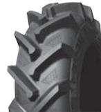
Specialized line for use on waterlogged and marshy terrain. The extremely deep lugs, together with the structure of the casing, provide high traction and flotation.
