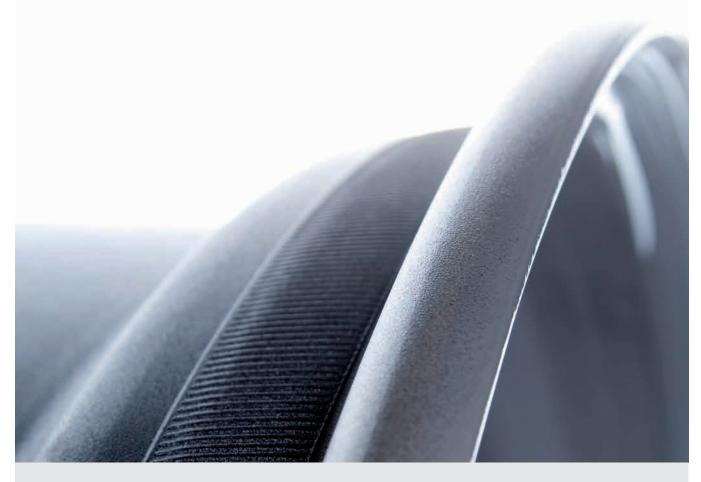
The knurling has been increased by 50% compared to the standard version. This, combined with the special black paint, maximises the friction characteristics of rim when the tire is fitted.
