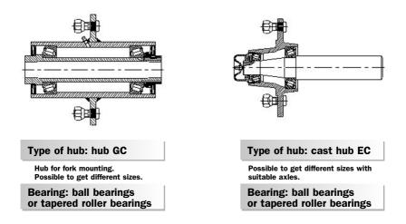
The axles produced are designed to match the hub of the wheel and the construction on which the axles are mounted.
