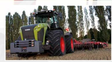
JJ and TH Haylock replaced a conventional tractor with an equal-wheeled, four-wheel steer Claas Xerion 5000, specifying Trelleborg High Power TM900s for maximum traction.
