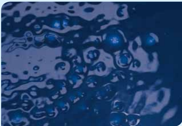
Paint flaws, such as these, are a result of contamination in the painting process.
