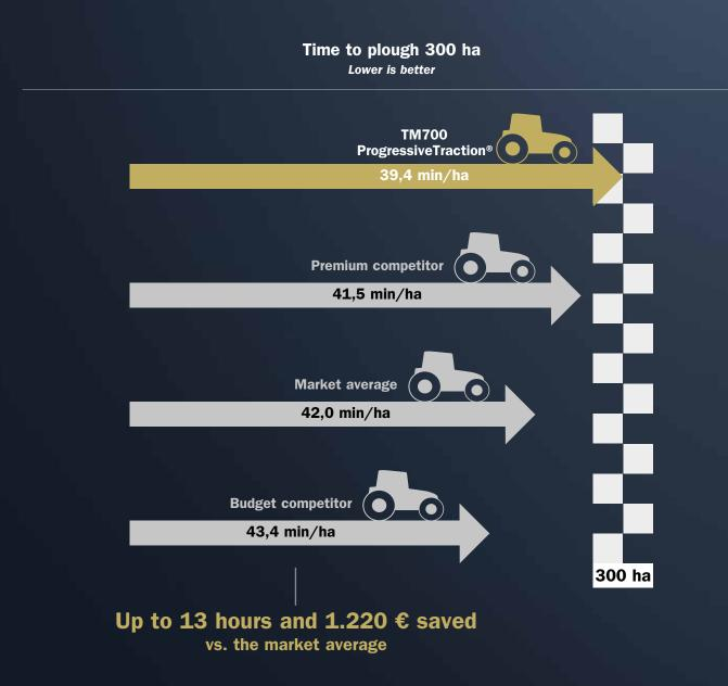
Soil condition: 40% sand, 35% loam, 25% clay Humidity: 15% Slippage: 5% - 20% Average working costs per hour = 95 € Including cost evaluation related to the tire wear performance
