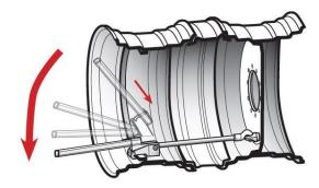
8. When the big clamp is open, cut off excessive length of the dual hook bar 20mm from the M20 nut
