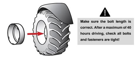
2. Align the drive disc with the assembled holder disc. Fasten the drive disc with the 12 enclosed bolts and washers. Tight to 365 Nm.
