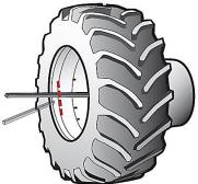
5. Roll, lift and align the outer wheel system close to the tractor. Make sure the tractor wheel is a little higher than the outer wheel.
