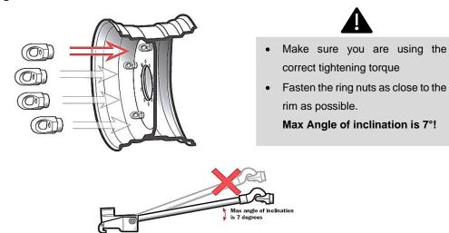
2. Fasten the dual hook bar with the big clamp, and then fasten the M20 nut at the end of the dual hook bar
