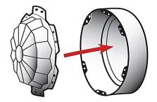
3. Mount the drum onto the disc of the outer wheel. Tighten to the recommended torque.
