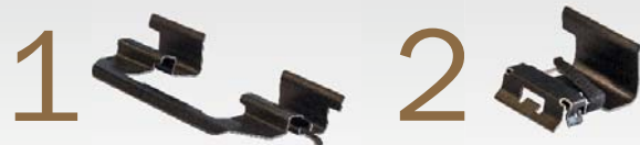
Abutment clips dampen the clunk or low-frequency noise by decoupling the pad ear, preventing in-plane energy from being transmitted to the calipers.
