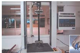
Determination of elongation at break at 20°C
