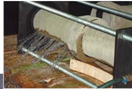
Water tightness test of the joint
