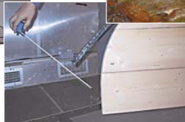
Determination of low temperature flexibility
