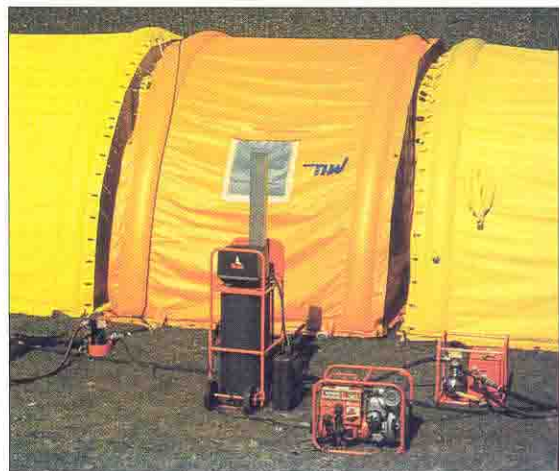
Hoses for fresh water and waste water are connected directly to the tent, giving a closed system.
