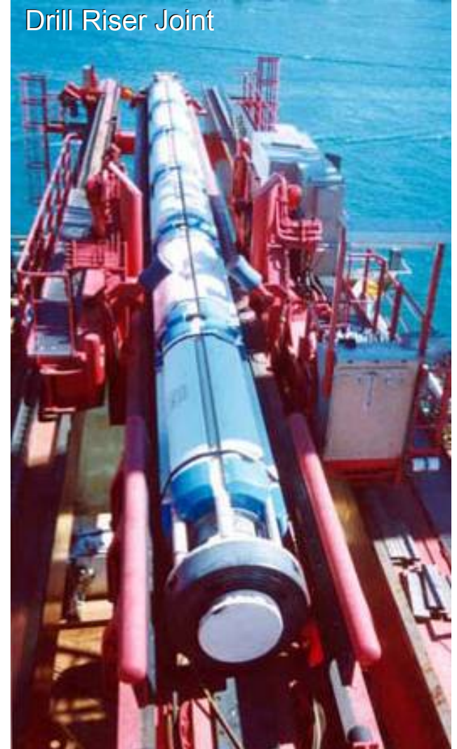
Drill Riser Pipe Joint being deployed
