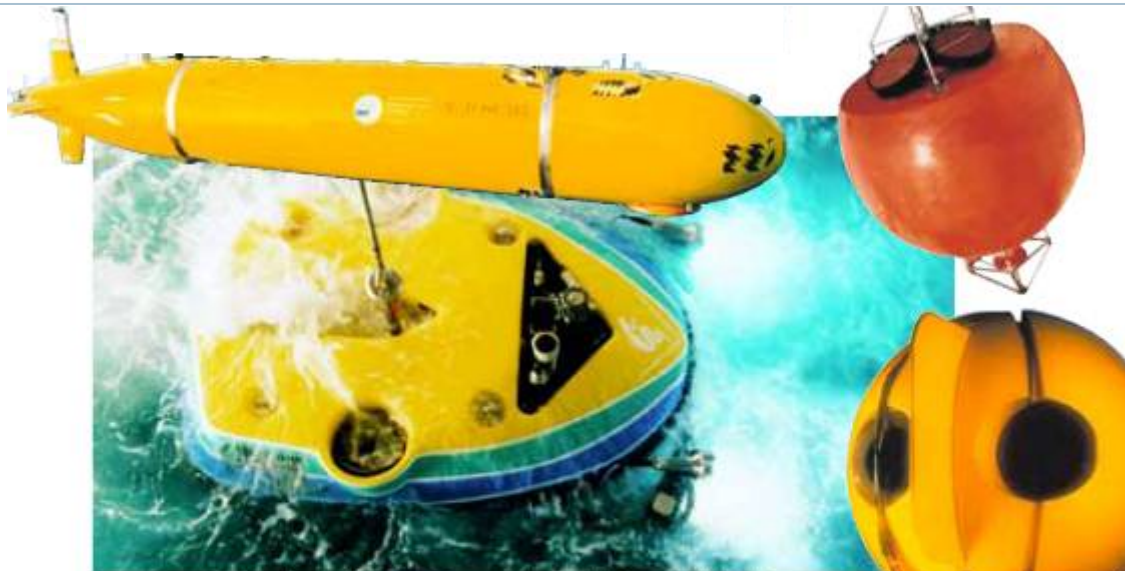
Top left to right: 2500 msw Autosub11, 1000 msw ADCP float Bottom left to right: 400 msw "Tiburón" (MBARI), Sonargraphic Buoy
